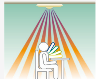
Quad element sensor to detect a small hand waving movement
